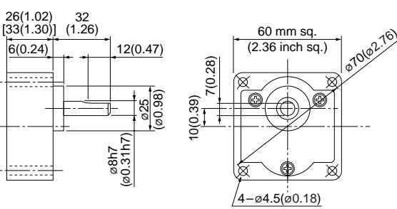
\* Figures in [ ] represent the dimensions of MX6G□B (M) (1/30 or larger reduction ratio).
