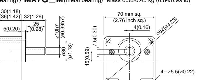
\* Figures in [ ] represent the dimensions of MX7G□B (M) (1/30 or larger reduction ratio).
